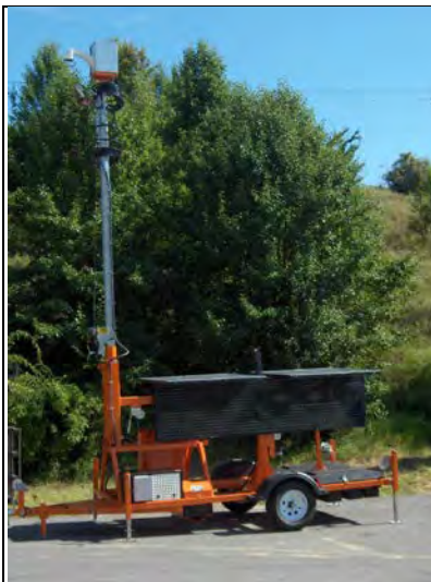
Figure 20 – Temporary DMS with CCTV Attachment
