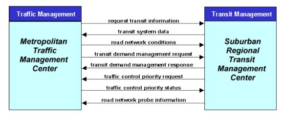
**Data Flow:** Representations of data flowing between processes or between a process and a terminator in the logical architecture of the National ITS Architecture. A data flow is shown as an arrow on a data flow diagram and is defined in a data dictionary entry in the logical architecture. Data flows are aggregated together to form high-level architecture flows in the physical architecture of the National ITS Architecture.
