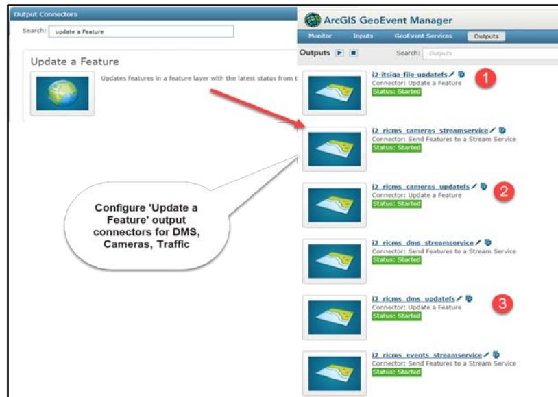
Figure 20 - 'Update a Feature' output connectors for DMS, Cameras, and Traffic data
