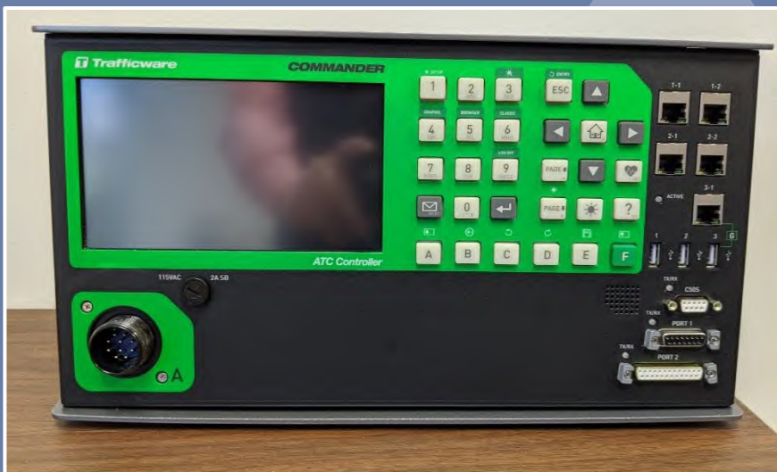
Trafficware (now Cubic ITS) COMMANDER ATC controller unit, NEMA TS-2, Type 1 model; shown in bench testing phase.
